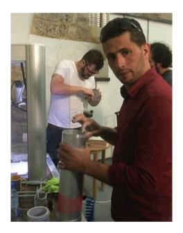
The clay for a 3D printer has to be fine, but can be exactly the same clay as for hand pottery. It needs to be mixed with water until it reaches a "nutellalike" consistency. Then the smooth clay mixture can be added to the 3D ceramic printer.
